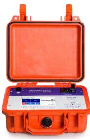
The instrument for measuring the electric resistance in the range within 10 mkOhm ÷ 10 kOhm on the currents of up to 10A:
