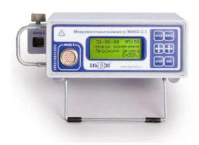
Operates in 4 modes: microohmmeter, milliohmmeter, kiloohmmeter and thermometer. MIKO-2.3 is a portable mini-laboratory allowing performing of all tasks connected with resistance measurement in electrical equipment as this instrument operates in four modes
