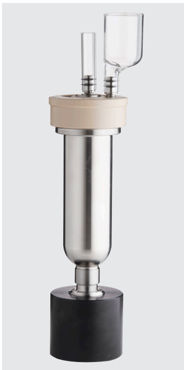
Fully assembled Test Cell in the assembly stand with glass fill and riser funnels.
